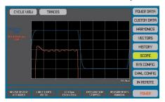
a full 10V square wave in blue and a 50:1 zoomed in view in red. Since the user sets amplitude and scaling - the result is an almost unlimited ability to amplitude zoom to expose fine detail. The sampling is forced to be asynchronous to higher order harmonics which leads to an effective sampling rate of 384MSPS.
